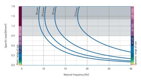
Natural frequency of a single-degree-offreedom system consisting of a fixed mass and an elastic bearing consisting of VIKAFOAM VF 950 on a stiff subgrade.
