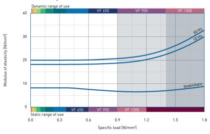
Dynamic test: sinusoidal excitation with an oscillating range of  $\pm\,0.22$  mm at 10 Hz and  $\pm\,0.08$  mm at 30 Hz
